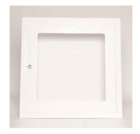
The hose cabinet is constructed in 16 gauge Cold Rolled Steel and comes with valve knockouts. Interior and exterior are treated with our exclusive WILCO "**PRO-TECH**" *Premiere* prime coating system. The door is fitted with 3/16" clear glass, stainless steel concealed latch and reinforced piano hinges.
